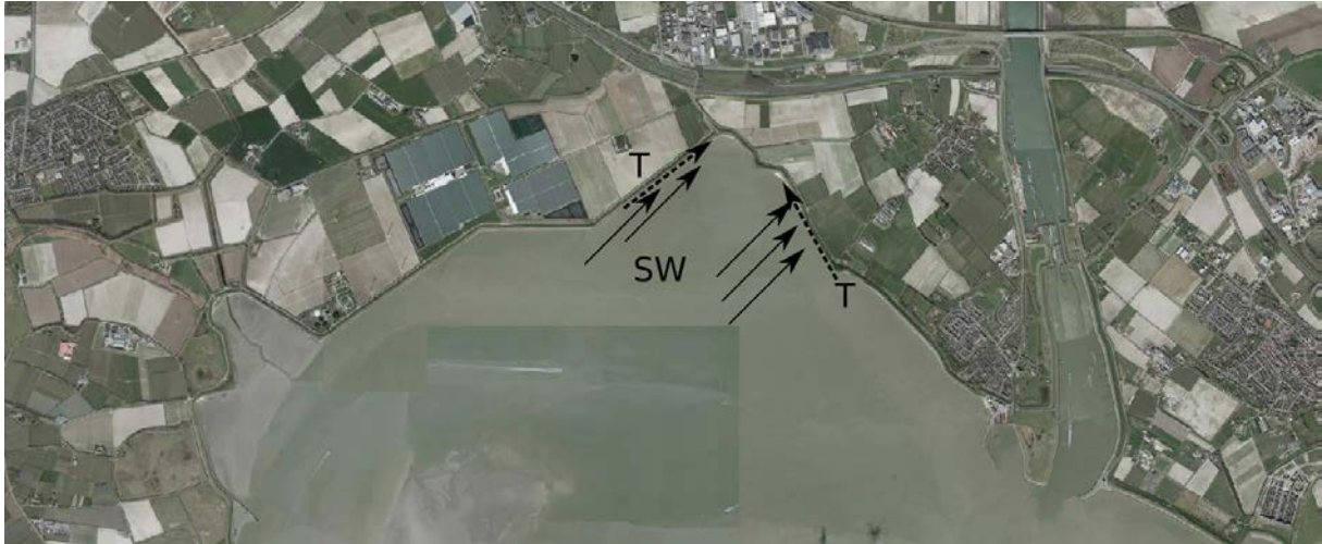
Illustration 1-9: Bank transport (T) with southwest winds on the North bank at Bath
