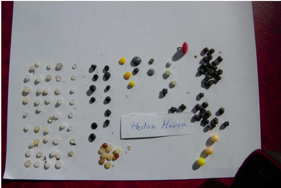
Nurdles Hedon Haven: the black, deteriorated, ones upper right (near thumbtack) are Bio Beads, the 3 balls down right are BB-Gun pellets (children's toy)
