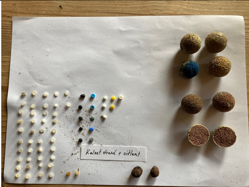
The 7 balls on the right are used to blow through (clean) the water pipes of power plants.
