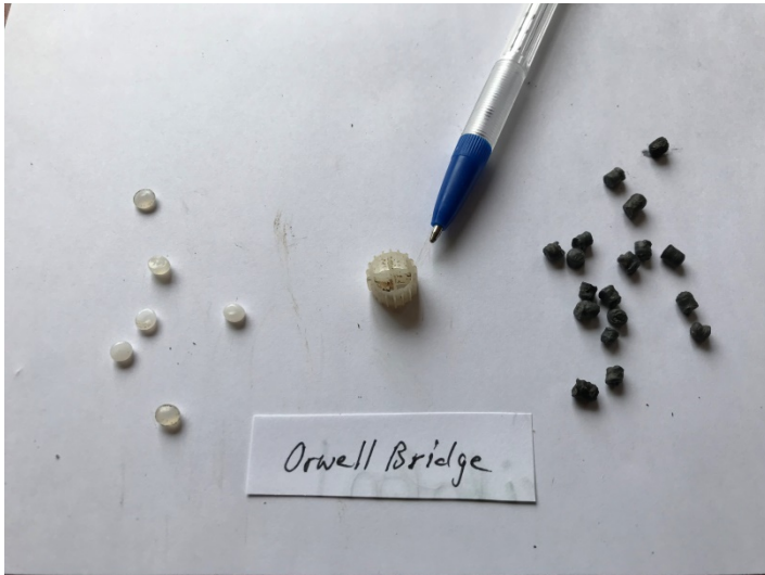
The wheel shaped plastic item indicated by the pen is also a bio medium which is used in waste water treatment Assisted Moving Bed (AMB) Bio Media | MBBR Wastewater Filter (dasusa.com)
