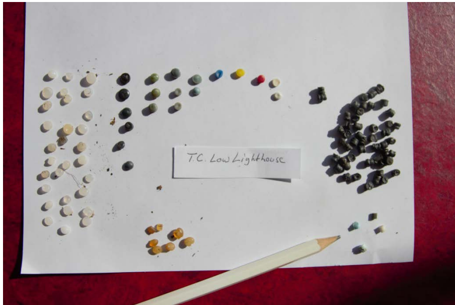
Nurdles Lighthouse: the black ones upper right are Bio Beads. The pencil points at cut of pieces of electrical wire
